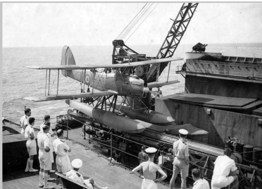
Catapult and hanger with Fairey Seafox Reconnaissance spotter seaplane mounted on H.M.S. Queen of Bermuda after modification at Newport News, Virginia, U.S.A.
